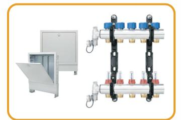
Manifold for the connection of the POLYMELT underfloor heating system or colling circuits with flowmeters in flow and automatic dynamic balancing valves in return for automatic hydraulic balancing. Made of stainless steel from 2 to 12 circuits available.
