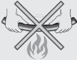
Thermoplastic material is flammable. Do not allow direct contact with fire PPR products!
