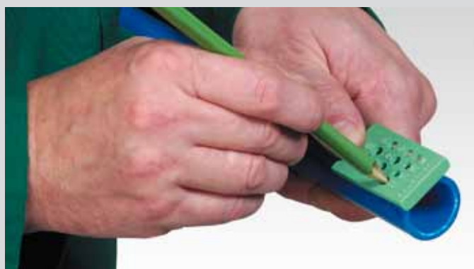
Marking of the welding depth
