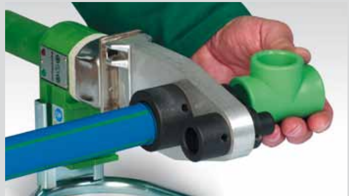
Heating-up of pipe and fitting
