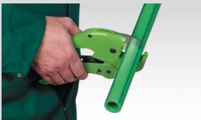
Cutting of the pipe
