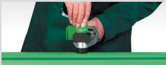
...heating-up of the elements
