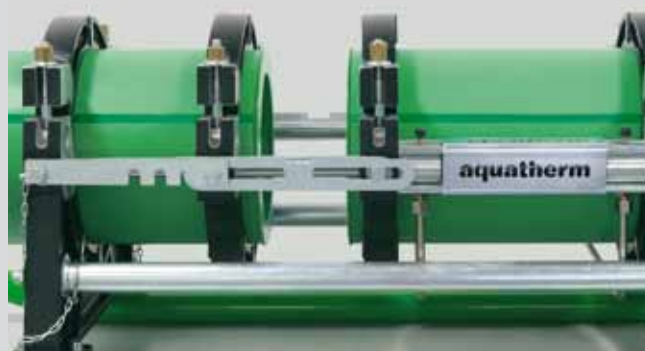
Divide the machine slide, remove heating element
