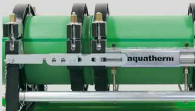
Join the pipes, cool down under pressure
