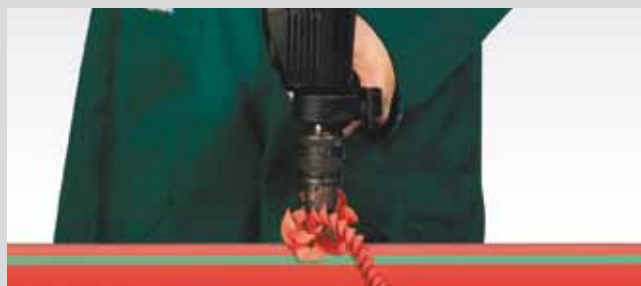
Drilling through the pipe wall
