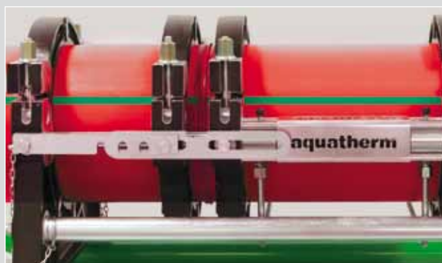
Join the pipes, cool down under pressure
