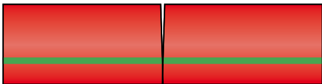
Gap width 160 mm outer diameter = 0.5 mm
