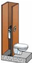
Installation with access from behind the wall
