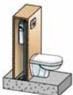
Installation on strong floor
