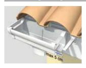
• Establish the position of the outlet and fit the end hooks at at least 50mm from the fittings to allow the gutter to expand freely.
