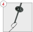
Slide the supporting clamp into the dedicated slit at the end of the rod.
