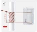
Decide where to position the collector on the downpipe. Then cut the pipe based on the length of the cutting template as shown on the back of the packaging. Remove the lower section of the downpipe.
